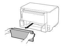
Put your hand on the handle of the maintenance box, and then pull the box outward.
