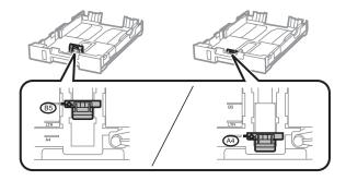
Load paper toward the edge guide with printable side face down, and check that the paper is not sticking out from the end of the cassette.
